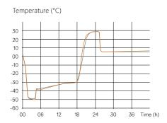
Example: Transfer of lyo-cycle from freeze-dryer A (24 m<sup>2</sup> / 258 sqft) to freeze-dryer B (33 m<sup>2</sup> / 355 sqft)
