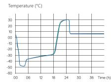
Lyo-cycle temperature profiles from different runs on both freeze-dryers are superimposed to demonstrate that the lyo-cycles are equivalent.
