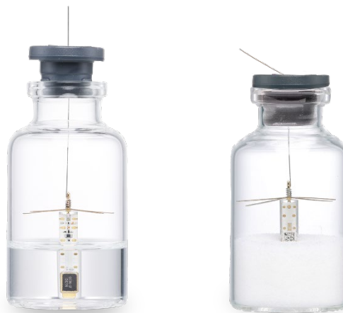
Figure 3.2-1: Sensor position in the vial before and after stoppering
